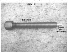
• Apply anti-seize to the 5/8" rod on the first 3 inches of thread from the alignment pin side of the rod (See fig. #2) DO NOT SKIP THIS STEP!!.
