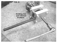
• The pulley may take quite a bit of force to remove. It is common to hear a *pop* when the pulley breaks free. Continue tightening the 5/8 rod until the pulley is removed. (We do not recommend the use of an impact wrench for this procedure; it usually damages the 5/8 rod and nut).
