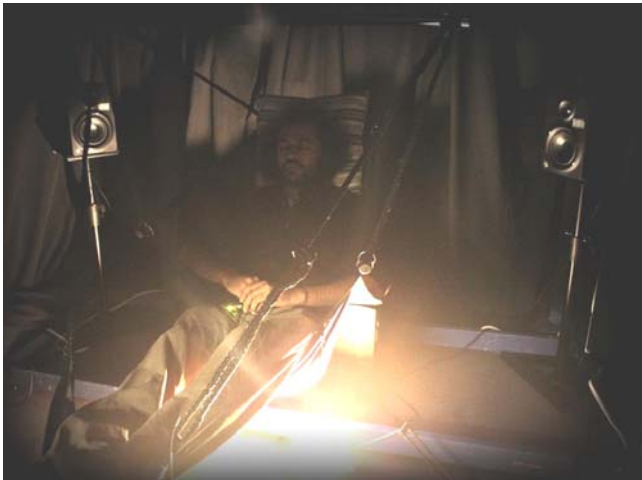
Figure 2. A user suspended in the Sonic Cradle . A light is turned on for documentation purposes; normally the room would be completely dark. Sensors detect the user's respiration and use this data to progressively shape a peaceful soundscape.
