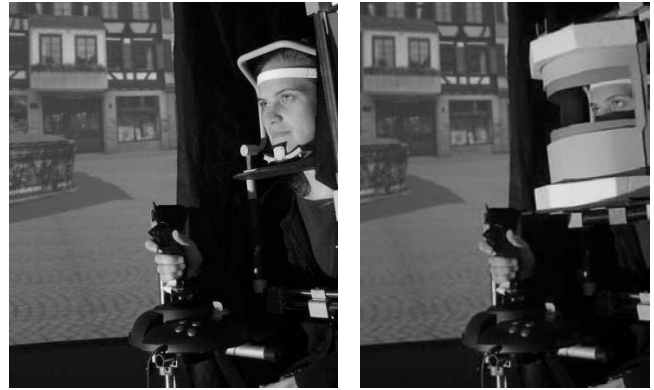
Figure 2: Full vertical FOV and restricted FOV setup in wheelchair
