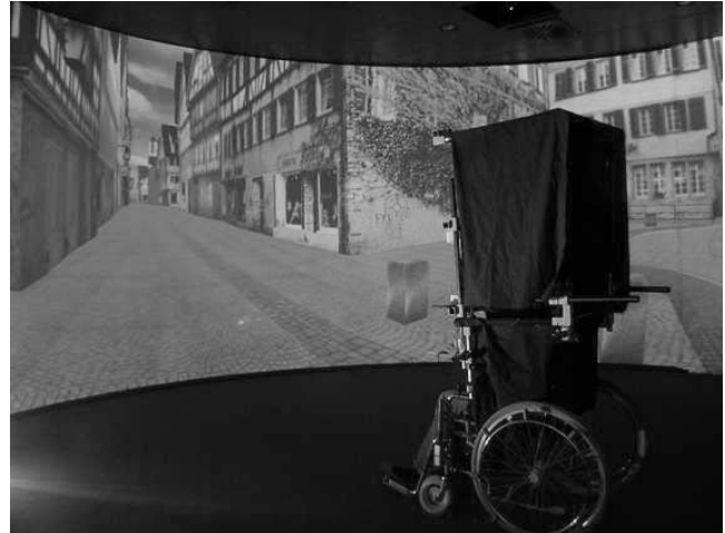
Figure 1: Wheelchair setup in front a large projection screen with a 3-dimensional model of a 280 meter street in Virtual Tübingen
