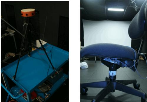
**Figure 1:** (a) Panoramic video capturing system. It includes 8 cameras mounted on a trolley which carries a PC and batteries for powering the cameras and the PC. (b) Interactive chair interface for supporting body based rotations in the panoramic view; a regular office chair has been modified by attaching an optical mouse to its rotating pivot. The mouse detects user's rotations in 360 degrees and the display system displays the corresponding part of the panoramic view.
