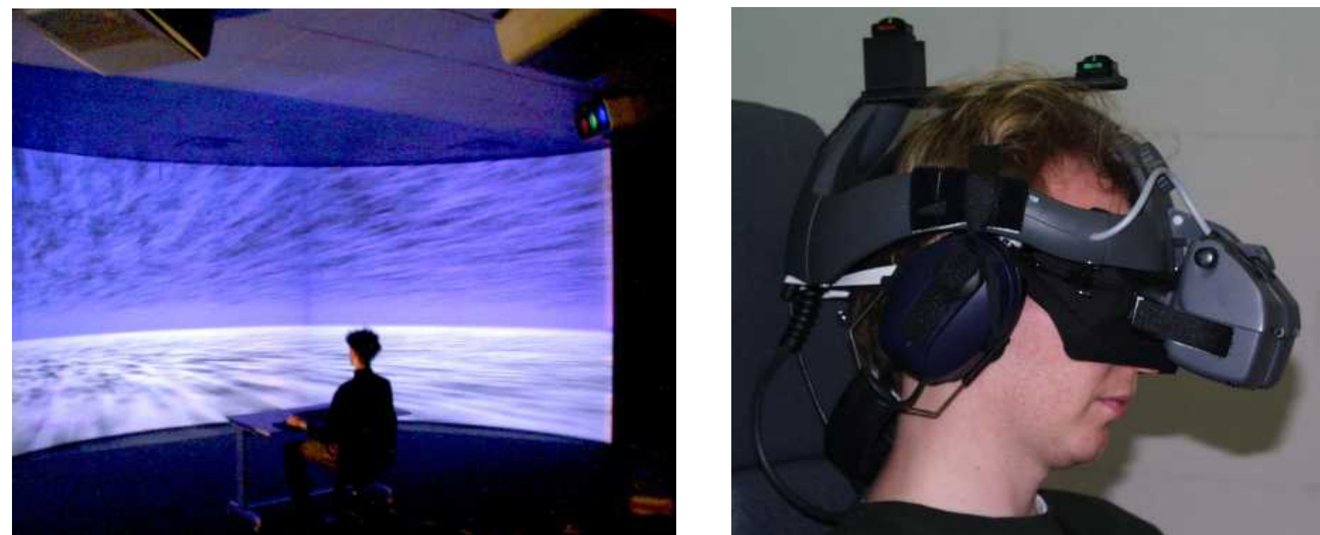
Figure 1: 180° half-cylindrical projection screen and HMD (FOV 40°x30°)
