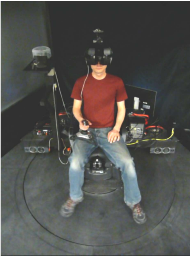
Figure 1. Experimental setup, showing the seated stationary participant stepping along the rotating circular treadmill. The head-mounted display (HMD) depicts the visual stimulus in the visual-only and bimodal conditions. For the biomechanical-only condition, the HMD was switched to black and participants were instructed to close their eyes. See included video or http://youtu.be/_vVqpWINF0 for an illustration of the three stimulus combinations. A handheld joystick was used to indicate the onset, intensity, and convincingness of the vection percept.
