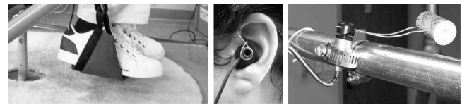
Figure 2: Left: Side view of the experimental setup, showing a participant with his feet suspended in the footrest attached to the hammock chair (“movement possible” condition). Center: Miniature microphones positioned at the entrance of the ear canals during the binaural recordings Right: A USB fan was modified to act as an eccentric motor that provided barely noticeable vibrations to the hammock chair.
