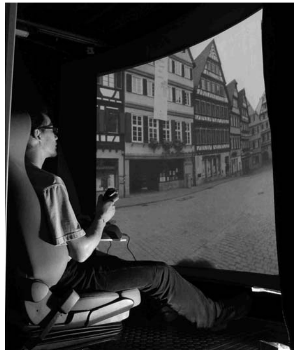
Figure 3: Participant seated in front of curved projection screen displaying a view of the Tübingen market place. The simulated FOV matched the physical FOV of 54°x40.5°.
