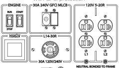
NEUTRAL BONDED TO FRAME NEUTRE MIS A LA MASSE A LA CARCASSE DU MOTEUR
