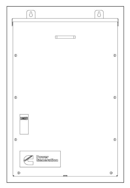
FIGURE 33. RA412N3 NON-SERVICE ENTRANCE TRANSFER SWITCH MODEL
