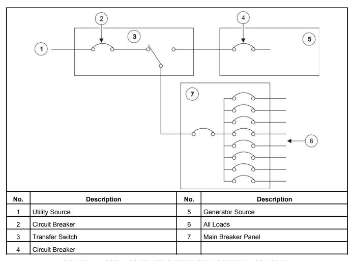
FIGURE 18. TOTAL COVERAGE SYSTEM (SERVICE ENTRANCE MODEL)
