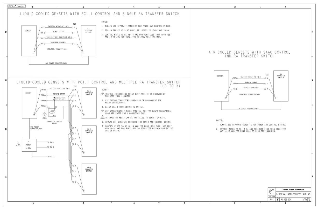
FIGURE 48. RA412N3 AND RA412S3 TRANSFER SWITCH INTERCONNECTIONS (SHEET 2 OF 2)
