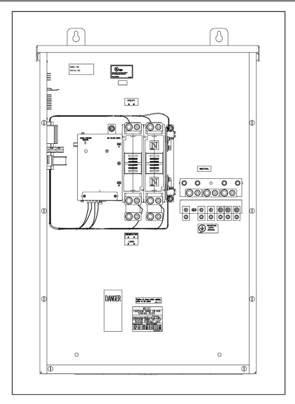
FIGURE 2. RA412N3 NON-SERVICE ENTRANCE TRANSFER SWITCH (WITH DOOR PANEL REMOVED)
