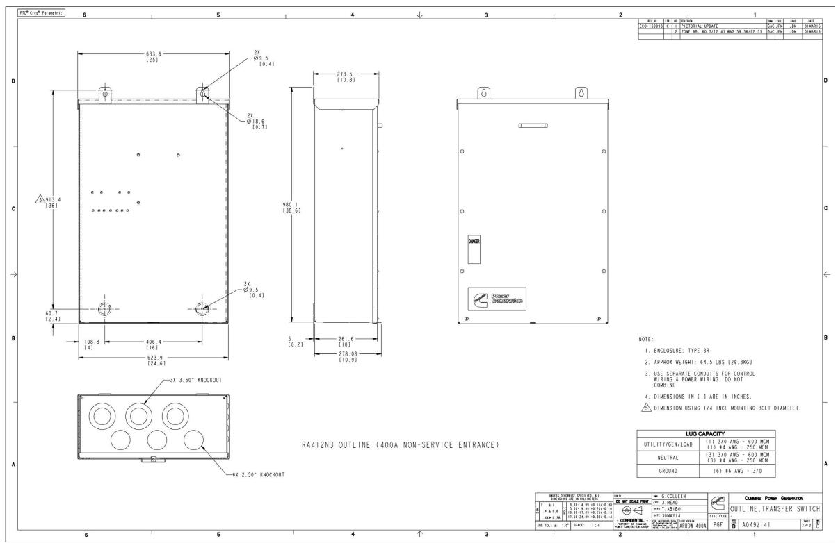
FIGURE 52. RA412N3 CONTROL BOX OUTLINE DRAWING
