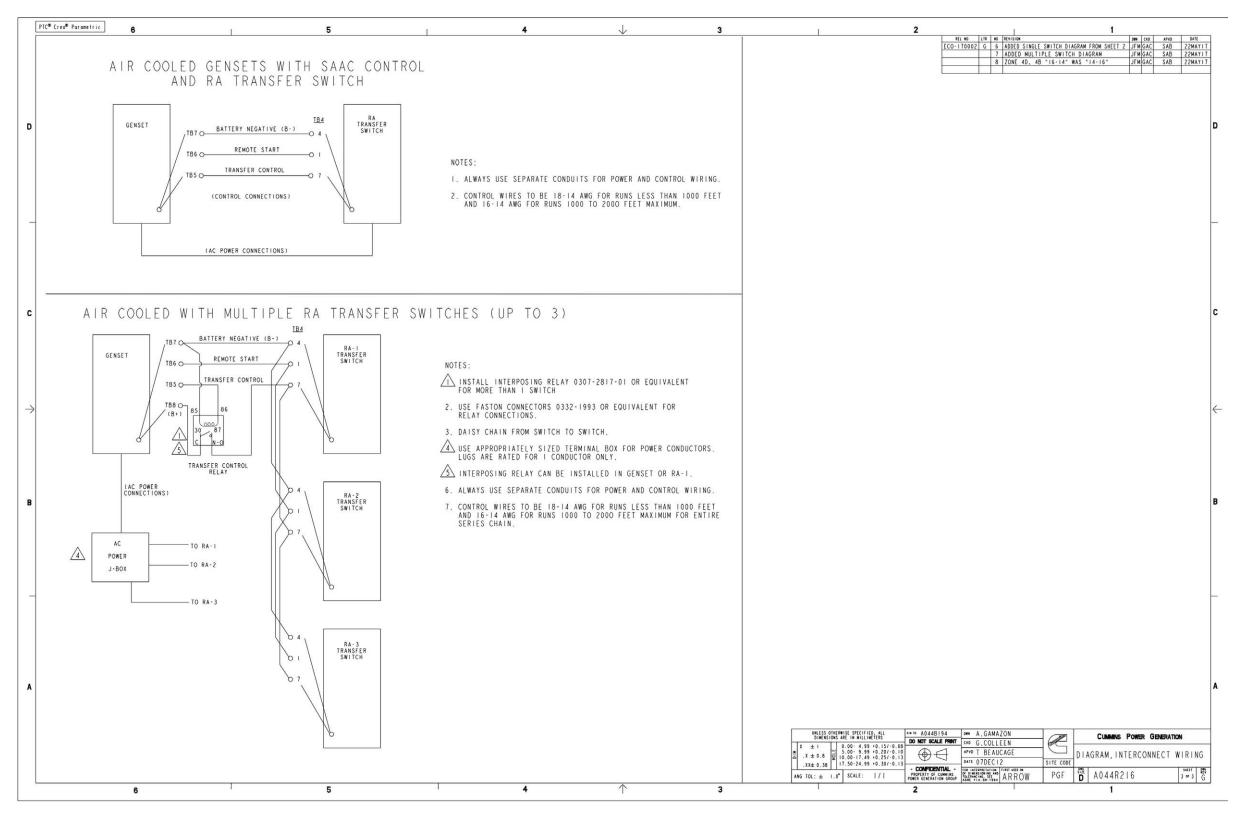
FIGURE 46. RA112N3, RA212N3, RA112S3, AND RA212S3 TRANSFER SWITCH INTERCONNECTIONS (SHEET 3 OF 3)
