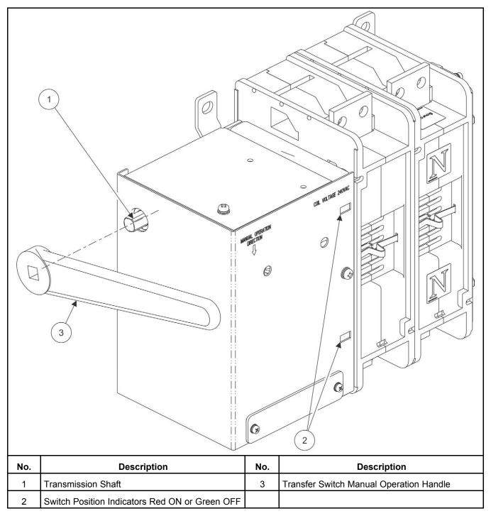
FIGURE 28. RA412N3 AND RA412S3 MANUAL OPERATION HANDLE
