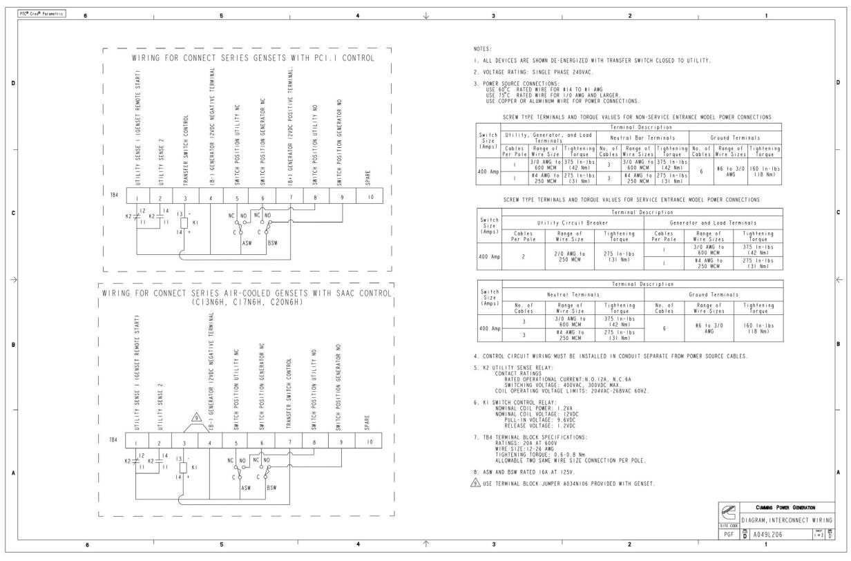
FIGURE 47. RA412N3 AND RA412S3 TRANSFER SWITCH INTERCONNECTIONS (SHEET 1 OF 2)
