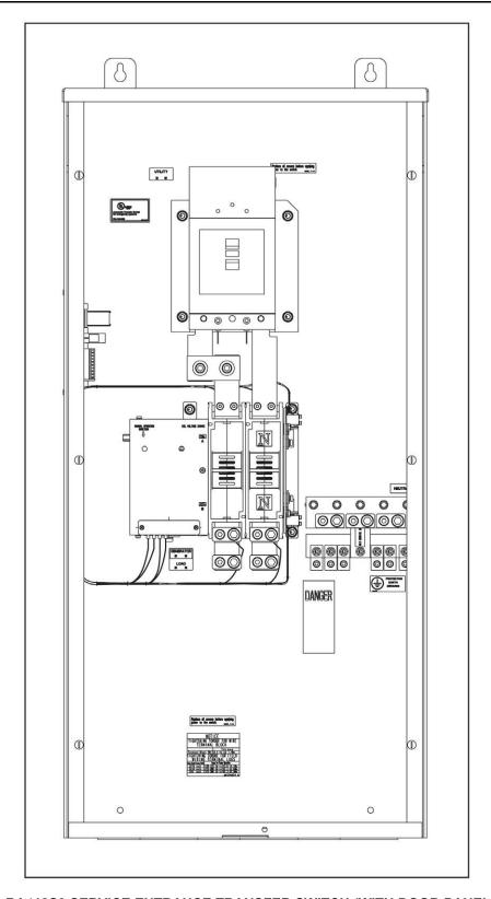
FIGURE 4. RA412S3 SERVICE ENTRANCE TRANSFER SWITCH (WITH DOOR PANEL REMOVED)
