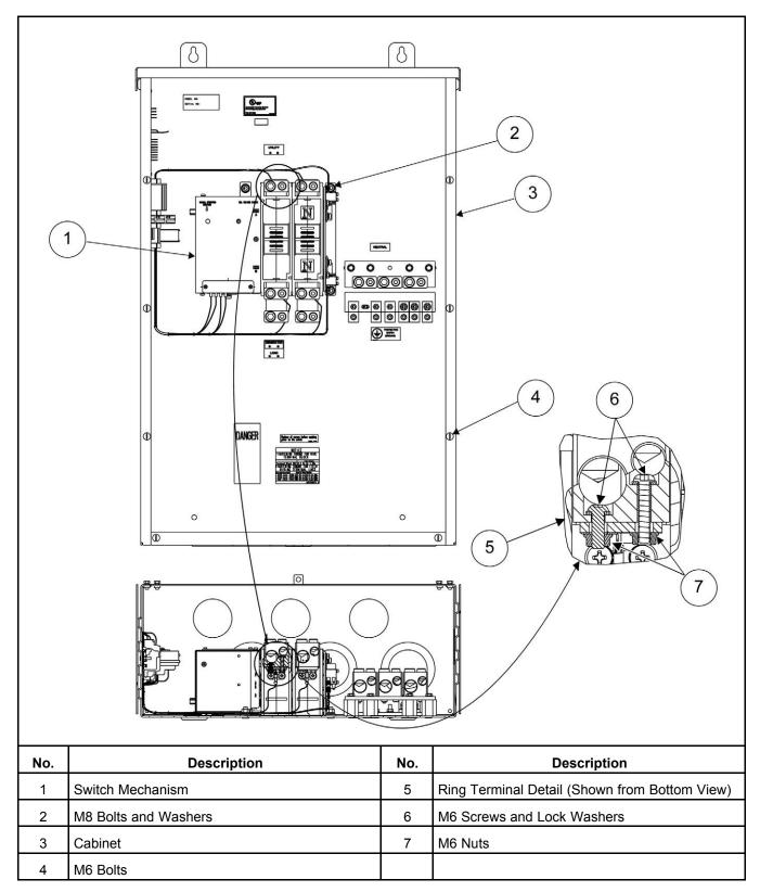
FIGURE 22. INTERIOR COMPONENTS FOR RA412N3 NON-SERVICE ENTRANCE MODELS
