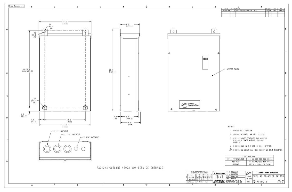
FIGURE 50. RA212N3 CONTROL BOX OUTLINE DRAWING
