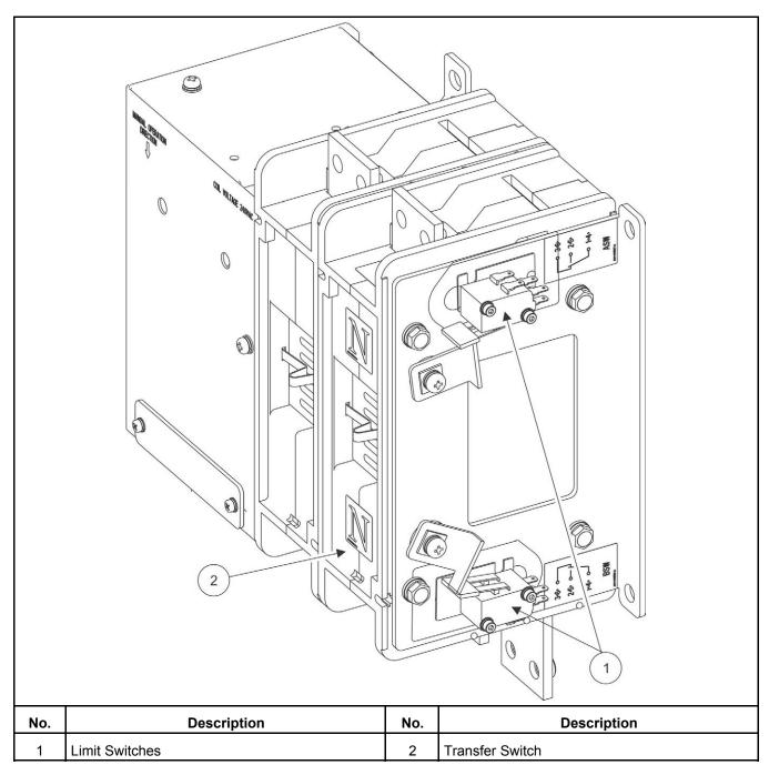
FIGURE 26. RA412N3 AND RA412S3 TRANSFER SWITCH REMOVAL
