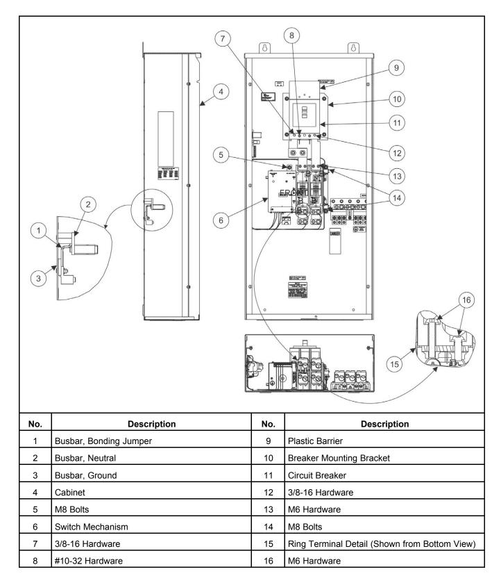
FIGURE 24. INTERIOR COMPONENTS FOR RA412S3 SERVICE ENTRANCE MODELS
