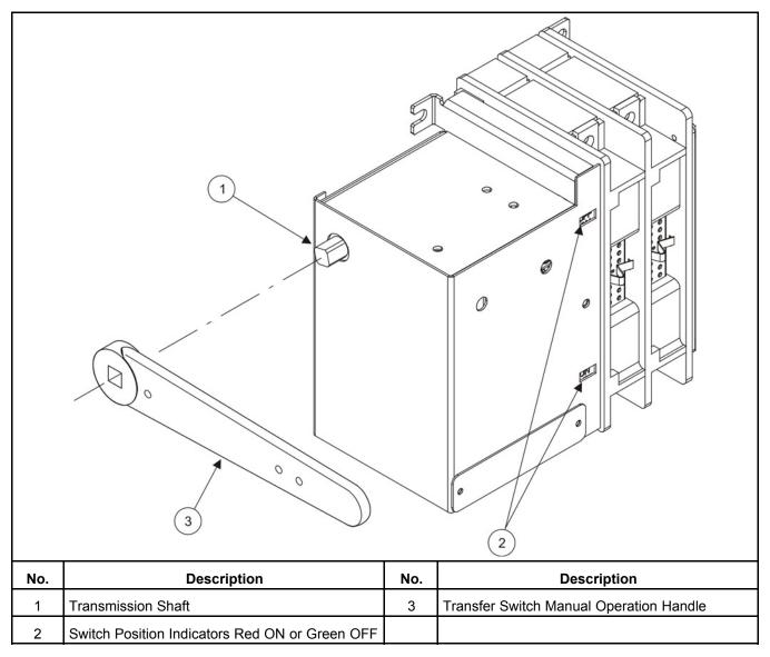
FIGURE 27. RA112N3, RA212N3, RA112S3, AND RA212S3 MANUAL OPERATION HANDLE
