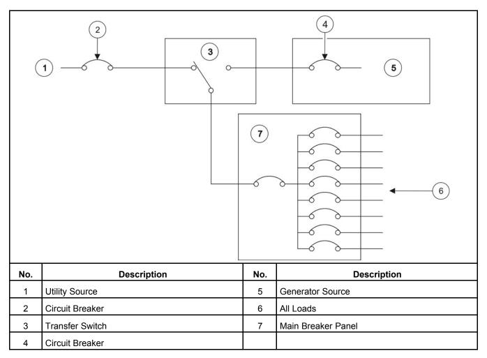
FIGURE 16. TOTAL COVERAGE SYSTEM (NON-SERVICE ENTRANCE MODEL)
