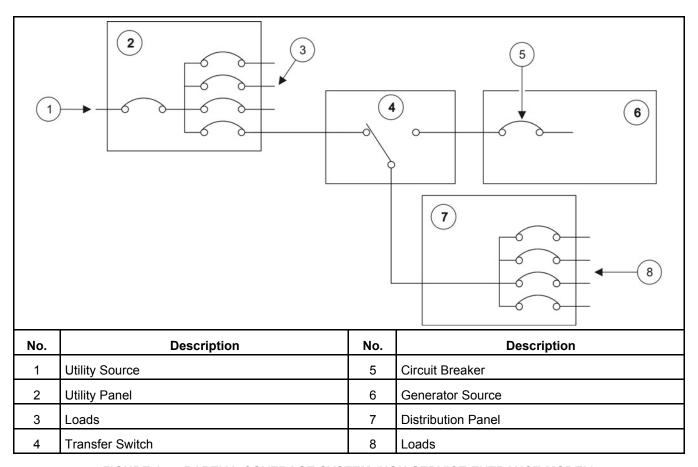
FIGURE 14. PARTIAL COVERAGE SYSTEM (NON-SERVICE ENTRANCE MODEL)
