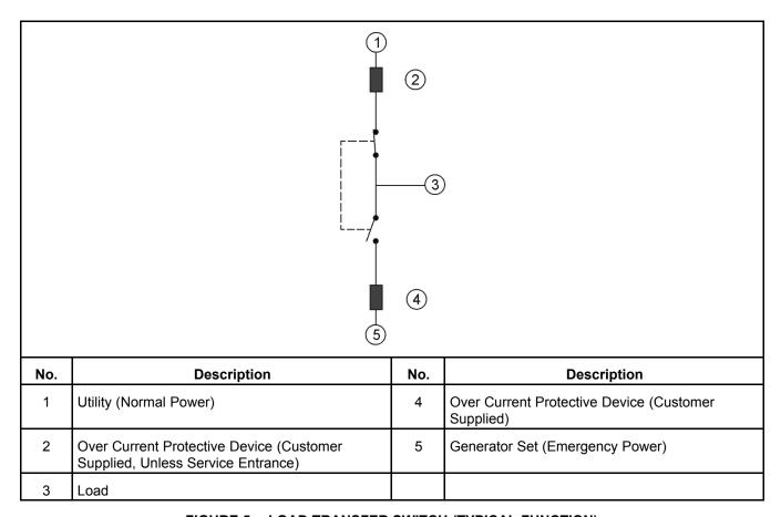
FIGURE 5. LOAD TRANSFER SWITCH (TYPICAL FUNCTION)
