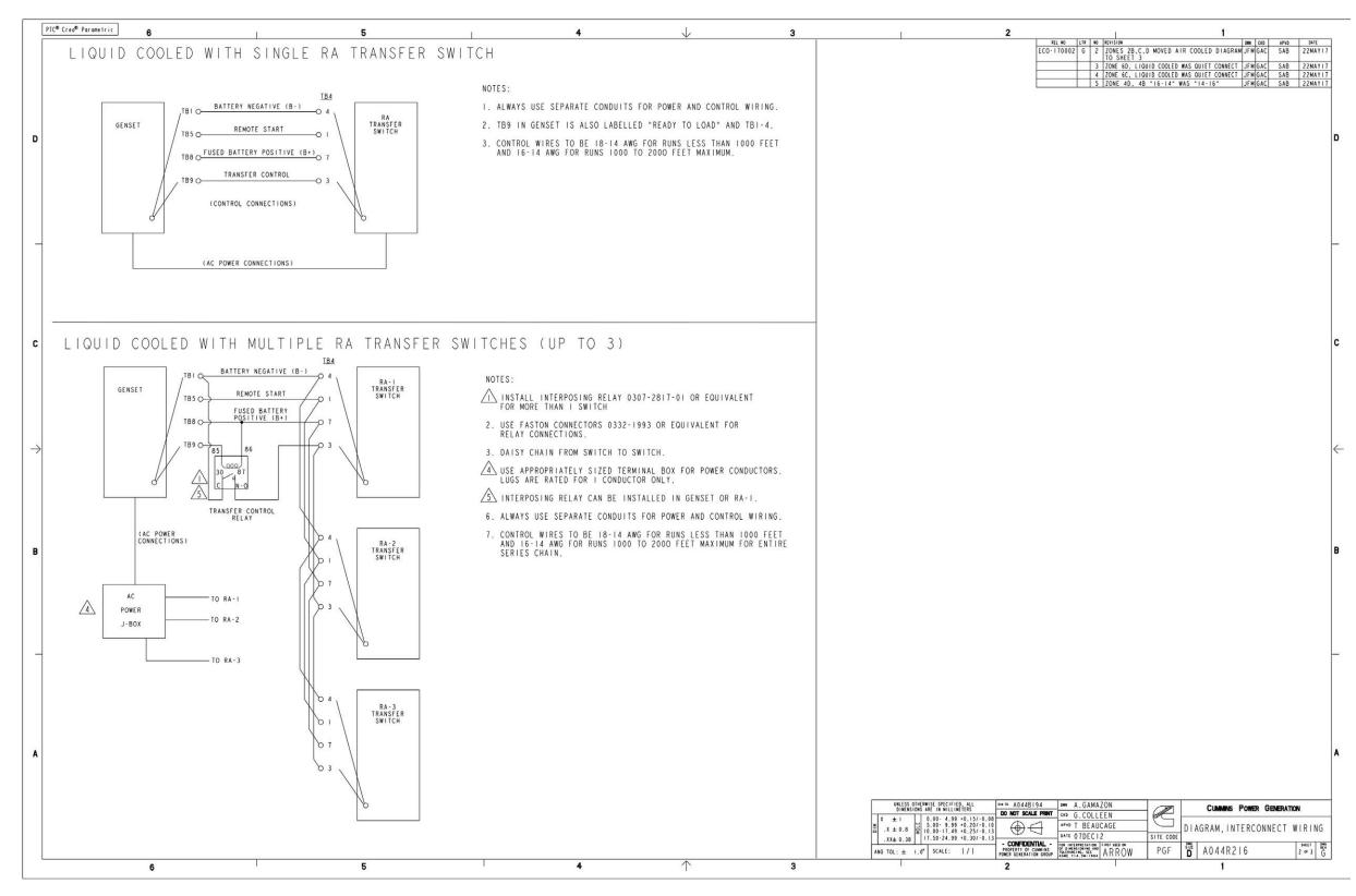
FIGURE 45. RA112N3, RA212N3, RA112S3, AND RA212S3 TRANSFER SWITCH INTERCONNECTIONS (SHEET 2 OF 3)
