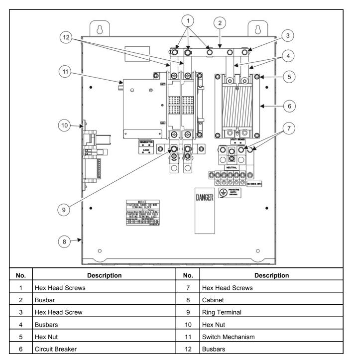
FIGURE 23. INTERIOR COMPONENTS FOR RA112S3 AND RA212S3 SERVICE ENTRANCE MODELS
