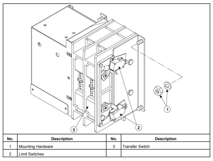
FIGURE 25. RA112N3, RA212N3, RA112S3, AND RA212S3 TRANSFER SWITCH REMOVAL
