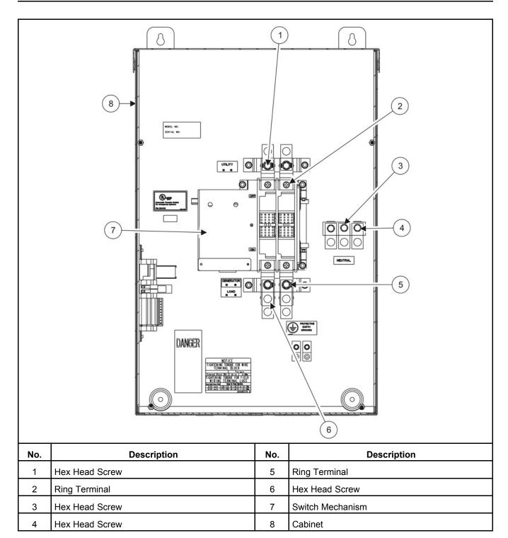
FIGURE 21. INTERIOR COMPONENTS FOR RA112N3 AND RA212N3 NON-SERVICE ENTRANCE MODELS
