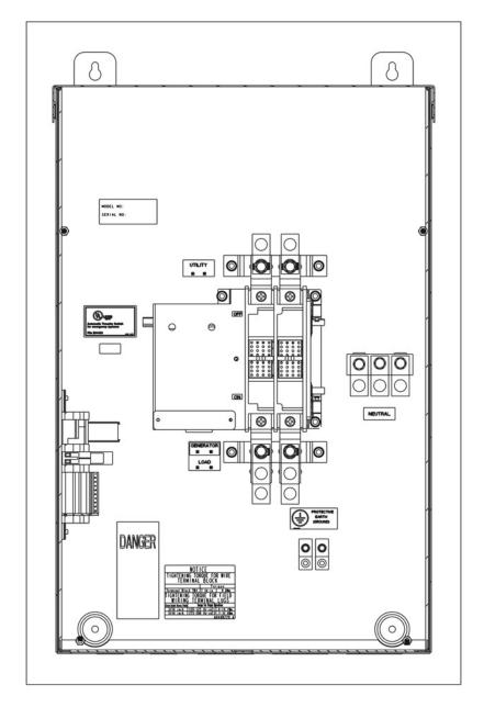
FIGURE 1. RA112N3 AND RA212N3 NON-SERVICE ENTRANCE TRANSFER SWITCH (WITH DOOR PANEL REMOVED)
