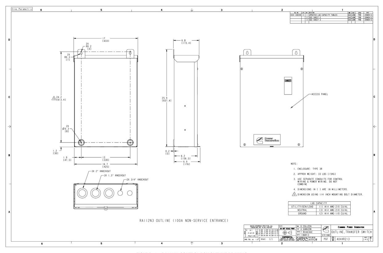
FIGURE 49. RA112N3 CONTROL BOX OUTLINE DRAWING
