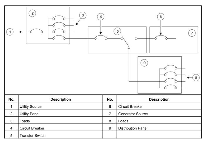
FIGURE 15. PARTIAL COVERAGE SYSTEM (SERVICE ENTRANCE MODEL)
