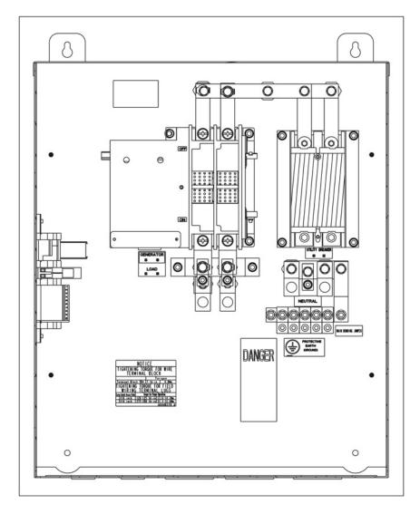
FIGURE 3. RA112S3 AND RA212S3 SERVICE ENTRANCE TRANSFER SWITCH (WITH DOOR PANEL REMOVED)
