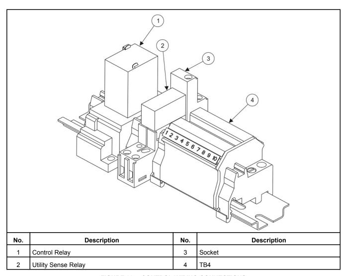
FIGURE 20. CONTROL WIRING CONNECTIONS
