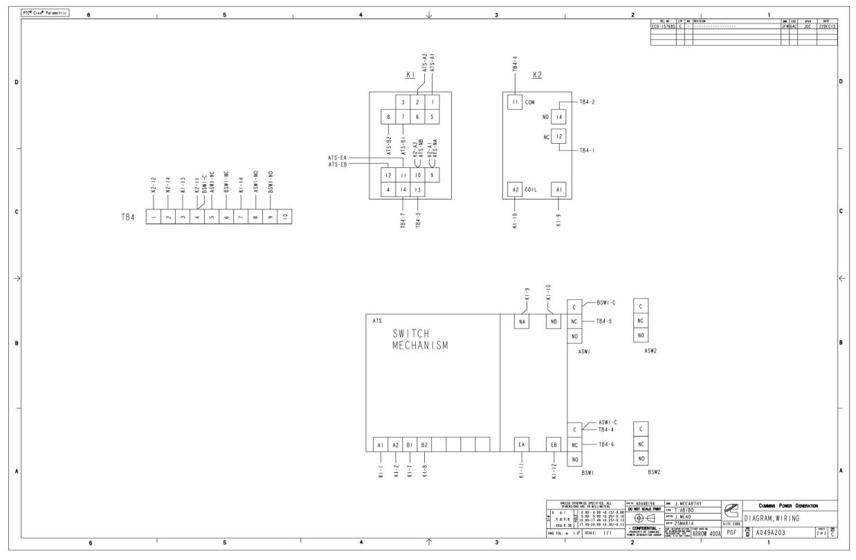
FIGURE 43. RA412N3 AND RA412S3 TRANSFER SWITCH WIRING DIAGRAM (SHEET 2 OF 2)
