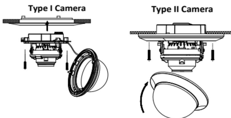
Figure 2-13 Fix the Camera to the Mount
