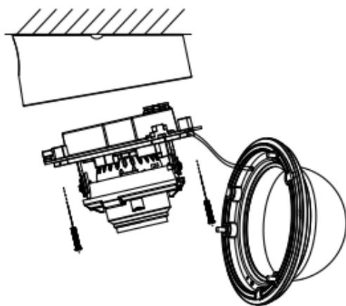
Figure 2-15 Fix the Camera to the Base
