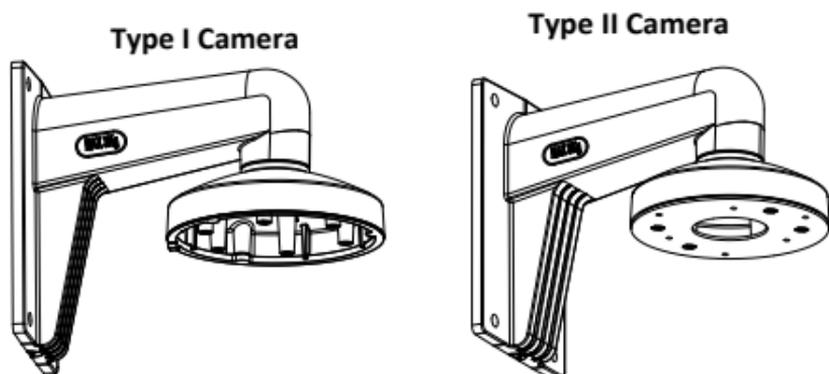
Figure 2-10 Install Wall Mounting Bracket
