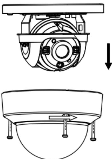
Figure 2-6 Remove the Bubble
