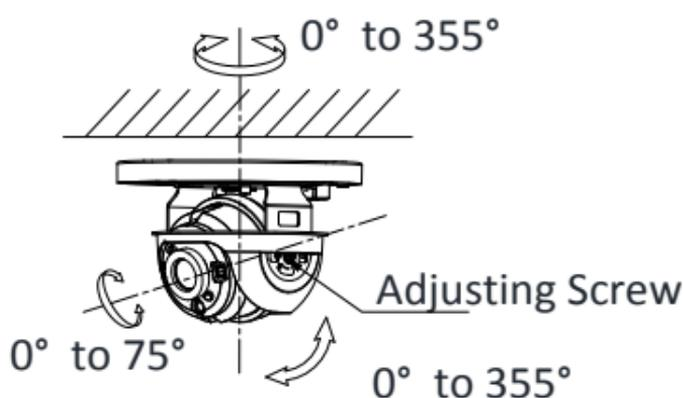
Figure 2-8 Type I Camera 2-Axis Adjustment
