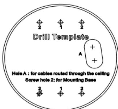
Figure 2-1 The Drill Template
