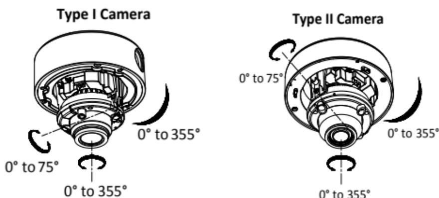
Figure 2-4 3-Axis Adjustment
