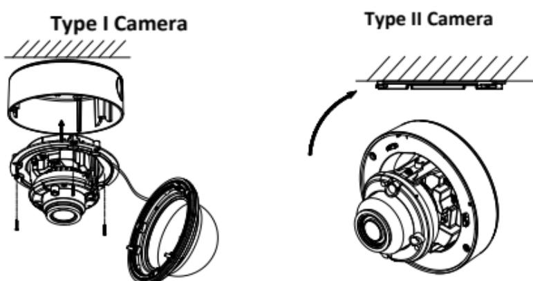
Figure 2-3 Fix the camera to the Ceiling
