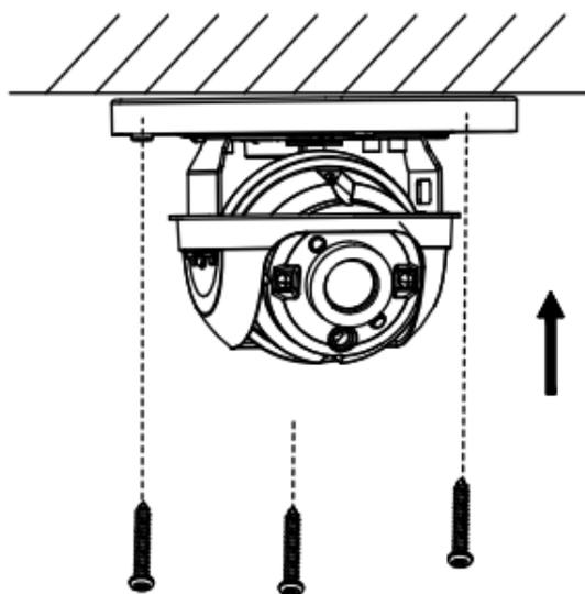
Figure 2-7 Fix the Mounting Base
