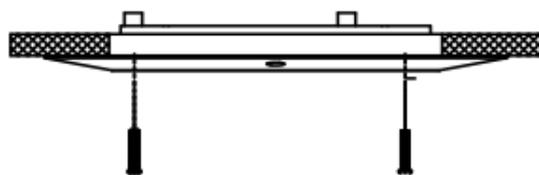
Figure 2-12 Install the In-Ceiling Mounting Bracket
