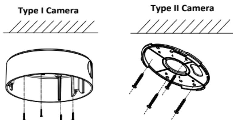
Figure 2-2 Attach the Back Box/Base Plate
