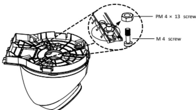
Figure 2-34 Secure Camera to Wall Mount Cover
