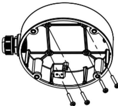
Figure 2-26 Secure Junction Box Body
