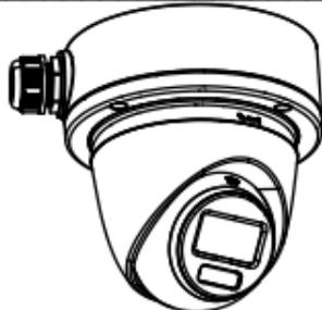
Figure 2-27 Combine Junction Box Cover with Body
