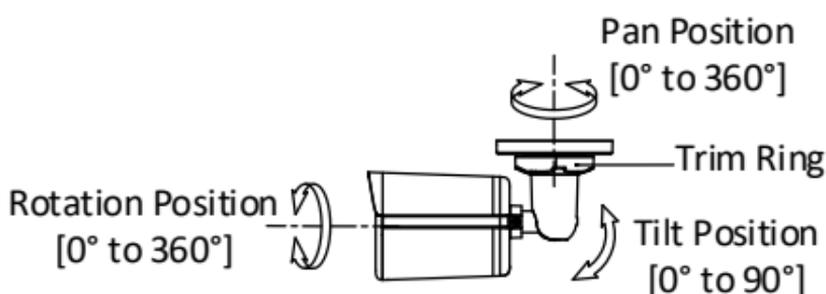
Figure 2-6 3-Axis Adjustment
