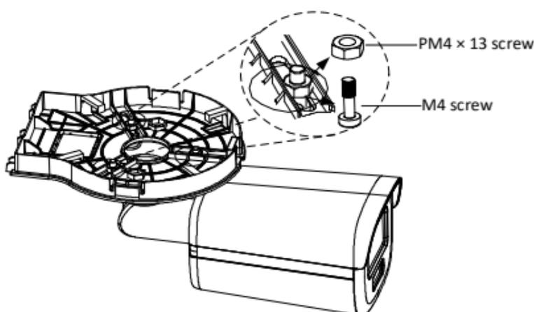
Figure 2-14 Secure Camera to Wall Mount Cover
