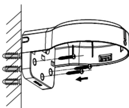
Figure 2-33 Secure Main Body to Wall
