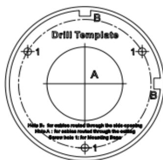
Figure 2-7 Drill Template for Junction Box
