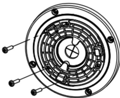
Figure 2-23 Install Installation Plate to Junction Box Cover
