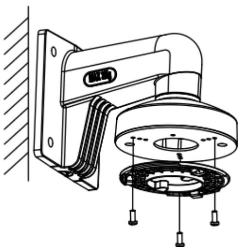
Figure 2-29 Fix Installation Plate
