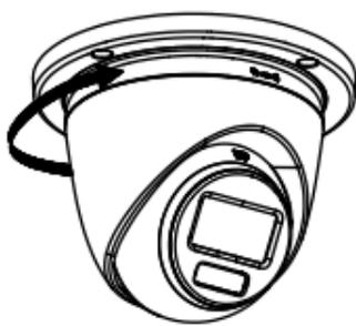
Figure 2-25 Snap Camera into Installation Plate
