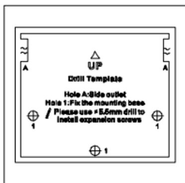
Figure 2-12 Drill Template for Wall Mount
