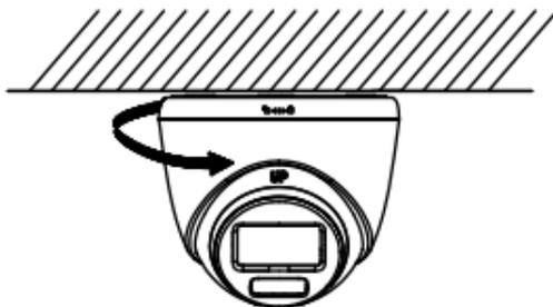
Figure 2-20 Snap Camera into Installation Plate
