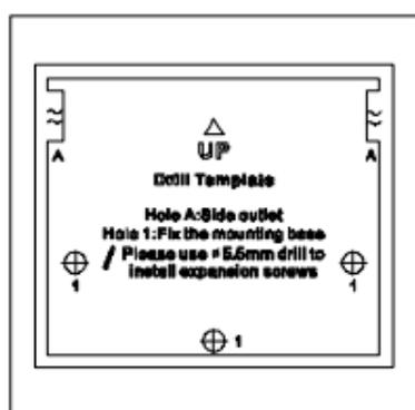
Figure 2-32 Drill Template for Wall Mount
