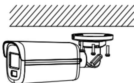
Figure 2-2 Secure Camera to Ceiling
