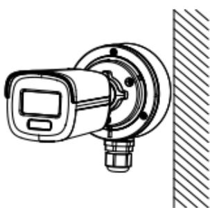
Figure 2-10 Fix Junction Box Cover on Its Body
