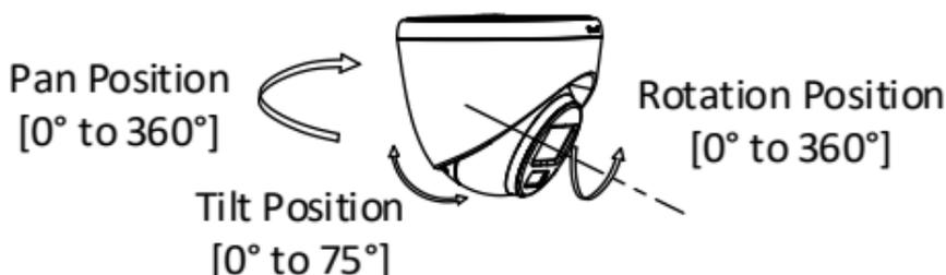
Figure 2-21 3-Axis Adjustment
