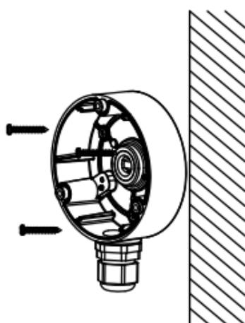
Figure 2-9 Secure Junction Box on Wall
