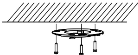
Figure 2-18 Attach Installation Plate to Ceiling
