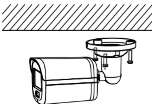
Figure 2-5 Secure Camera to Ceiling
