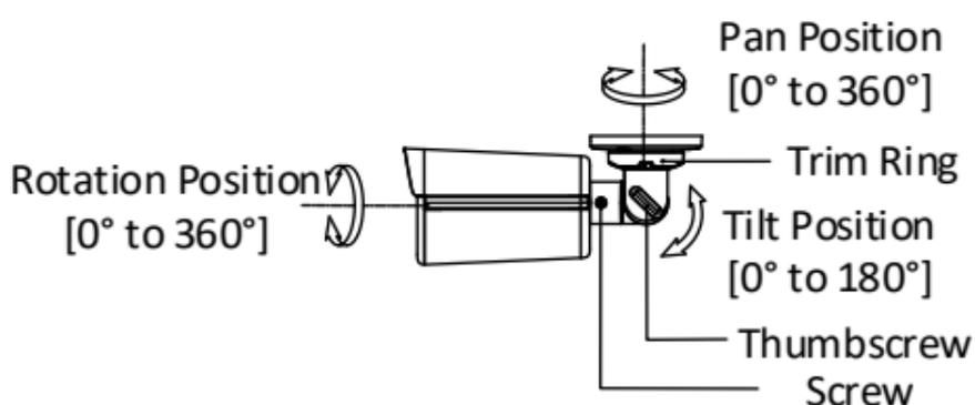
Figure 2-3 3-Axis Adjustment
