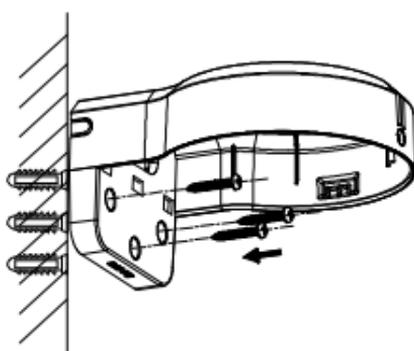
Figure 2-13 Secure Main Body to Wall
