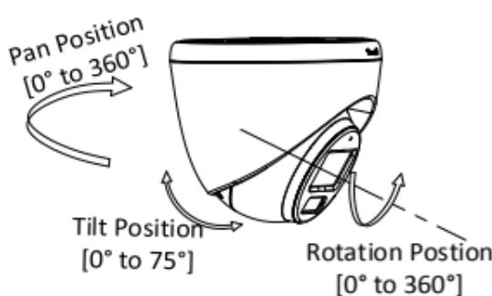
Figure 2-9 3-Axis Adjustment
