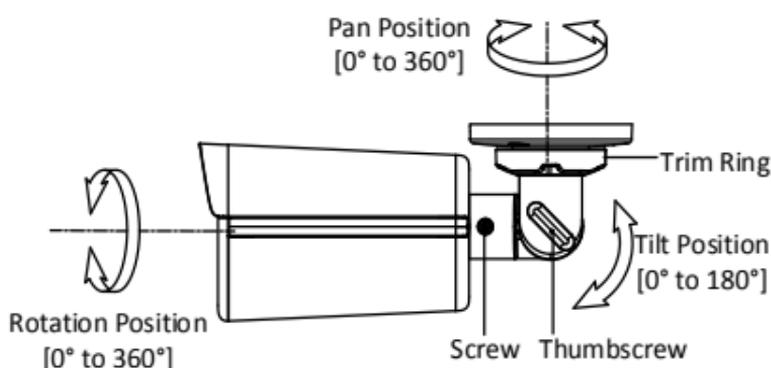
Figure 2-2 3-Axis Adjustment
