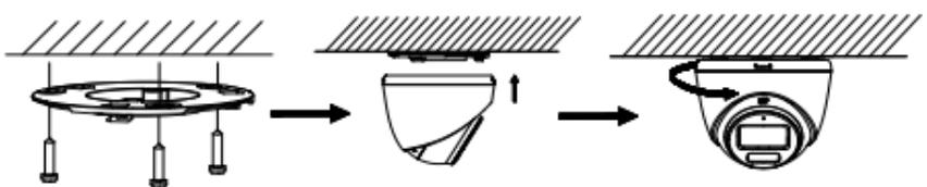
Figure 2-6 Install the Camera to Ceiling
