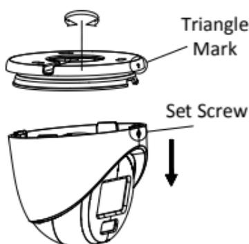
Figure 2-7 Disassemble the Camera
