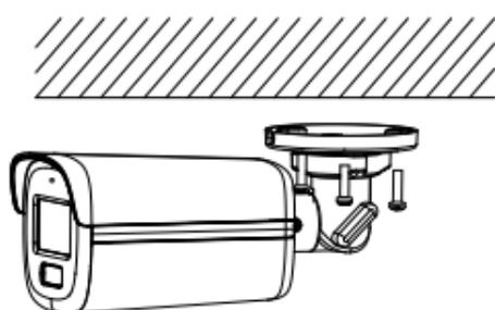
Figure 2-1 Secure the Camera to the Ceiling
