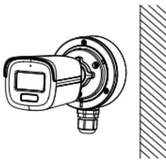
Figure 2-5 Fix the Cover to Its Body
