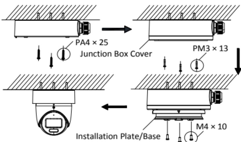
Figure 2-11 Fix the Camera to the Junction Box
