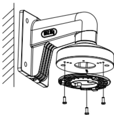
Figure 2-13 Fix the Installation Plate
