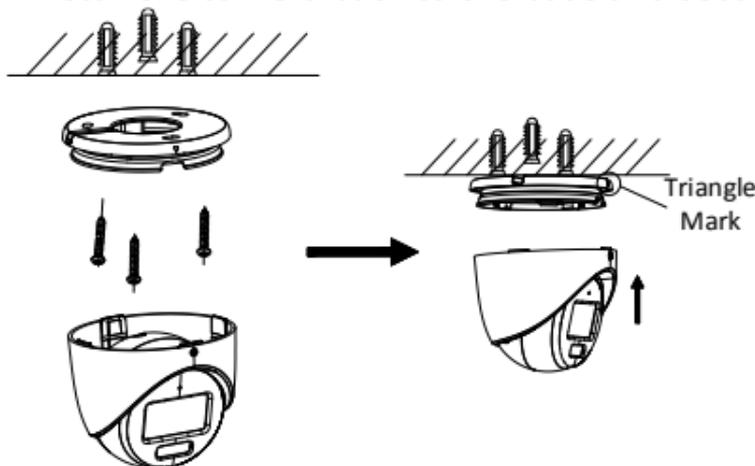
Figure 2-8 Install the Camera to Ceiling
