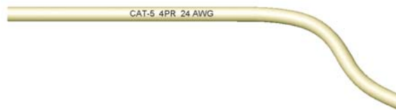
Figure 34: Straight and Even Cable
