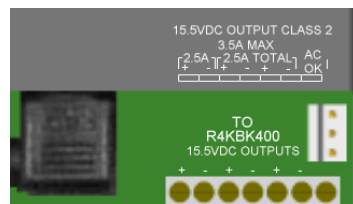
Figure 71: Power Supply outputs
