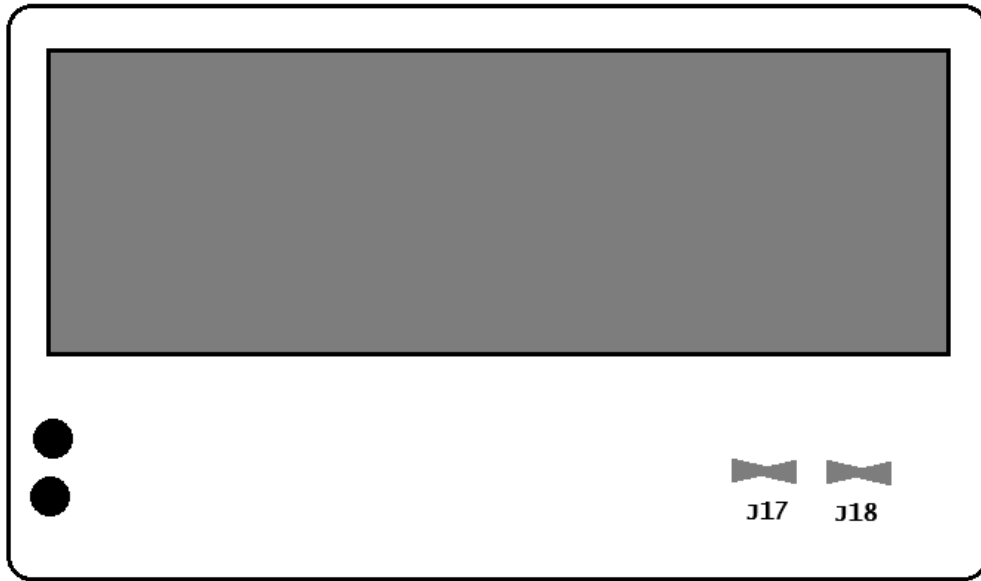
Jumpers J17 and J18 on the main board.
