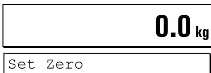
Set gross weight to zero (only within selected range for pushbutton zero)
