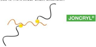
The chain extended polymer remains a mainly linear polymer with higher molecular weight
