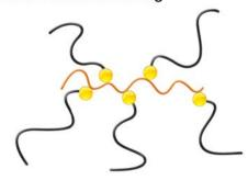
The chain extended polymer will contain some branched and higher molecular weight polymer chains
