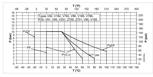
The pressure-temperature diagram is based on a lifetime of 25 years and water or similar media.
