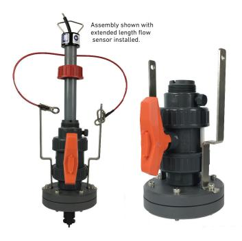
The Signet 3519 Flow Wet-Tap Valve serves as a unique interface between the installation fitting and the wet-tap style Signet 515 or 2536 Rotor-X flow sensor. It provides a fast method of removing the sensor from the pipe under specified operating pressures. The PVC and stainless steel design of the Wet-Tap makes it resistant to corrosion and chemical attack by acids, alkalies, salt, and a number of other harsh chemicals.
