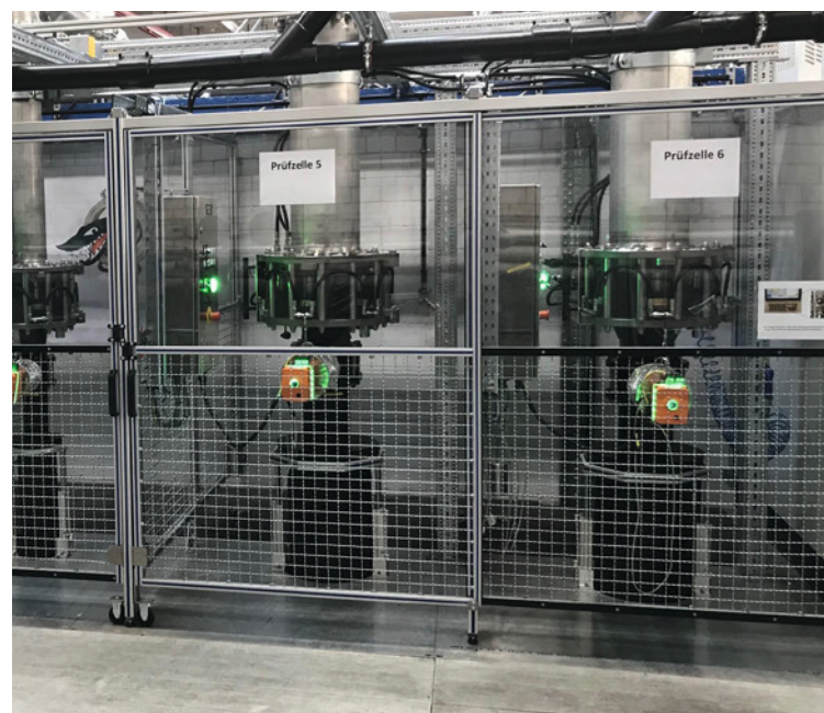
To ensure the high quality standard, the butterfly valves are tested under the toughest conditions in a test stand.
