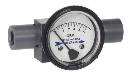
Plast-O-Matic flow gauges indicate liquid flow rates from low flows of 0-1 GPM to 0-10 GPM, even when used at high line pressures. Flow gauge sensors can be supplied with switches or relays to initiate alarms, activate other equipment, or shut the system down. Two switches are used when high and low limits are desired. Maximum line pressure rating is 200 PSI.
