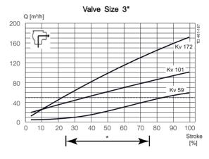
Alfa Laval recommend max. flow velocity in tubing and valves to be  $5\ \text{m/sec}$ .
