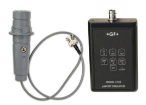
The Signet 2759 pH/ORP Simulator is a battery-powered millivolt generator that simulates pH values of 4, 7 and 10, plus ORP values of  $\pm 700$  mV. This device is useful as a troubleshooting aid and for general verification of system operation. It is not a substitute for periodic system calibration with pH buffers or test solutions.
