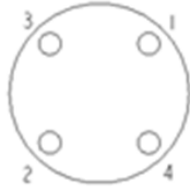
Fig. 5: Bolt Tightening Sequence
