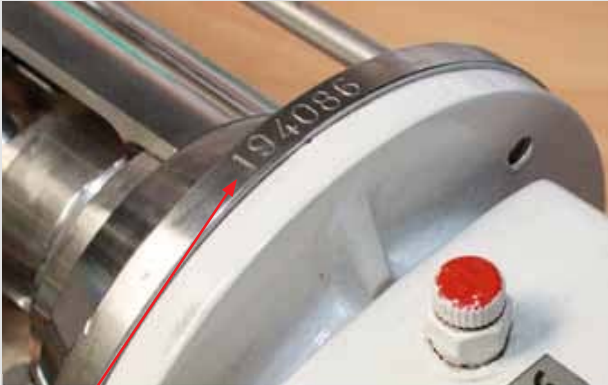
Serial ID number on the pump housing flange on the drive side
