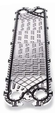
WideStream: Our WideStream plates with clip-on gaskets have very few contact points, which helps prevent blockage and results in longer uninterrupted operating times. Available only for Alfa Laval FrontLine, the plates are specially developed for the pasteurization of fruit juices and other products containing a limited amount of pulp and fibres.
