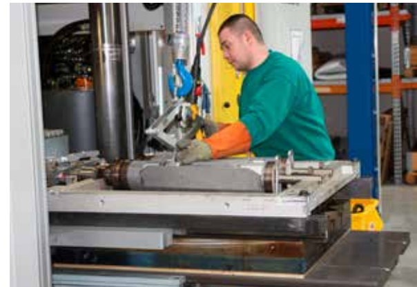
Injection molding machine for iFD-stators®
