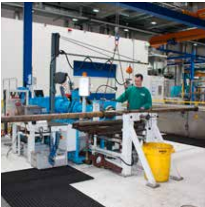
Extruder with stator for oil production
