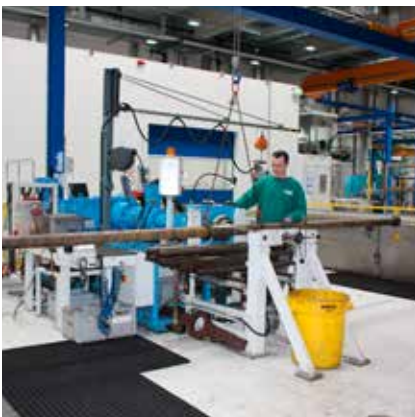
Extruder with stator for oil production
