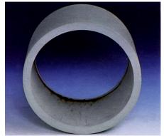
Fig. 3 PP Pipe, Standard Quality After Chromic Acid Test.
