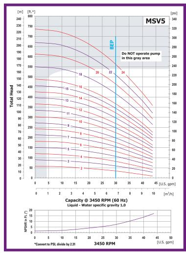
units designed to handle high-pressure low flow liquid transfer applications where no suction lift is required. Typical installations include: hot and chilled water, boiler feed, condensate return, irrigation, high pressure washdown, booster service, and fire protection/sprinkler systems—often referred to as a Jockey Pump. These pumps have NOT been investigated for use in potable (drinking) water systems.
