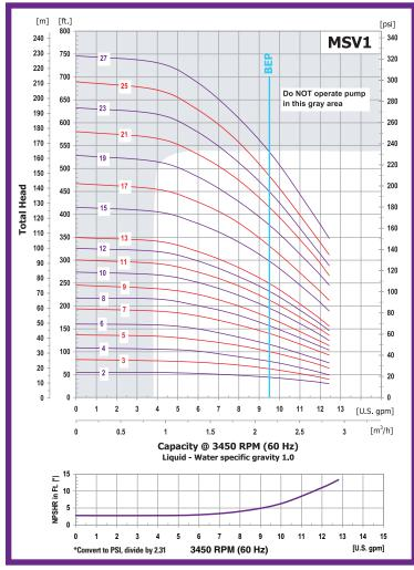
These AMT commercial/industrial centrifugal pumps are non-self-priming (gravity feed) units designed to handle high-pressure low flow liquid transfer applications where no suction lift is required. Typical installations include: hot and chilled water, boiler feed, condensate return, irrigation, high pressure washdown, booster service, and fire protection/sprinkler systems—often referred to as a Jockey Pump. These pumps have NOT been investigated for use in potable (drinking) water systems.
