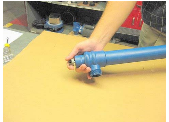
To install the impeller you will need to hold the pumps coupling...
