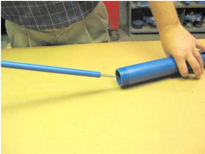
Insert outer tube over shaft assembly. The outer tube will want "hang up" on the guide bearing.
