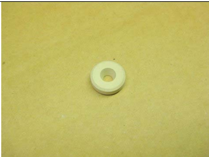
Top view of new seal (tapered side)
