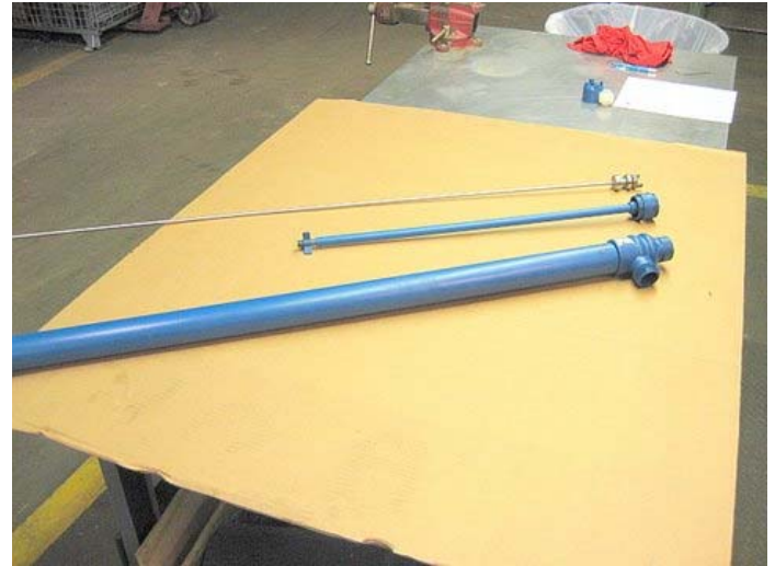
Picture illustrating shaft with bearing assembly, impeller housing with lower inner tube and center bearing removed from pump tube.
