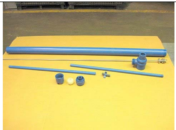
Picture illustrates pump completely disassembled.
