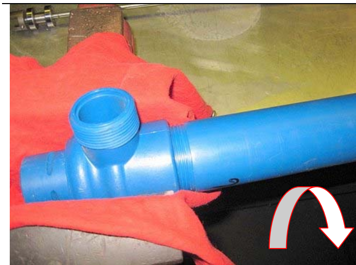
Place pump head in a vise and remove the intake tube by unthreading clockwise.
