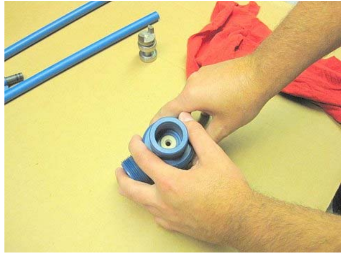
Using no larger than a 3/4" diameter rod, tap seal until fully seated in counter bore.
