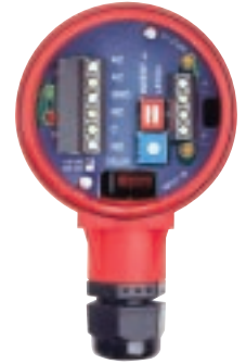
Compact Relay Controller (inside shown)
