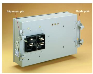
Well-made busway solutions come with thoughtful installation aids like the alignment pin on this bus plug, which prevents technicians from installing the device 180 degrees out of rotation.
