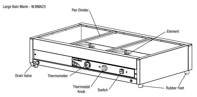
These bain maries may be used wet or dry, depending on the application. Once unit has been used as a WET bain marie it cannot be used dry as the elements will have absorbed moisture and water borne minerals which will affect the reliability of the unit should it be run dry.
