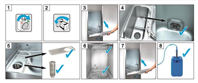
**IMPORTANT** Dosing devices must be primed when air gets into the dosing hose due to the containers not being exchanged or refilled in time (▶ 6.3.2).
