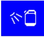
A display on the screen indicates when integrated storage tanks are empty (► 11.1). External storage tanks have to be fitted with a suction tube with level control if a display on the screen is required to show when the filling level drops.
