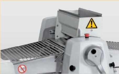
The automatic flour duster (option) dusts your dough band with flour precisely and evenly. This significantly minimises the amount of flour used.
