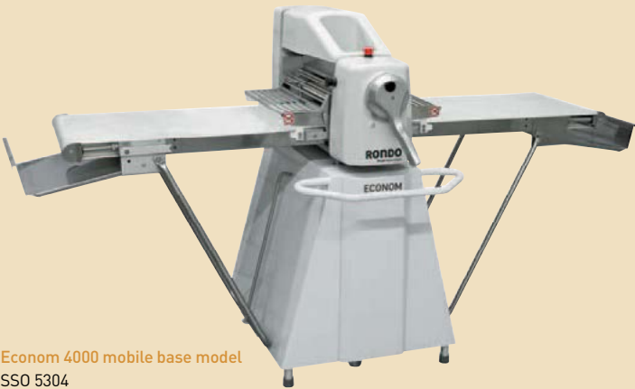
When not in use, the tables are simply folded up and you gain valuable working space.
