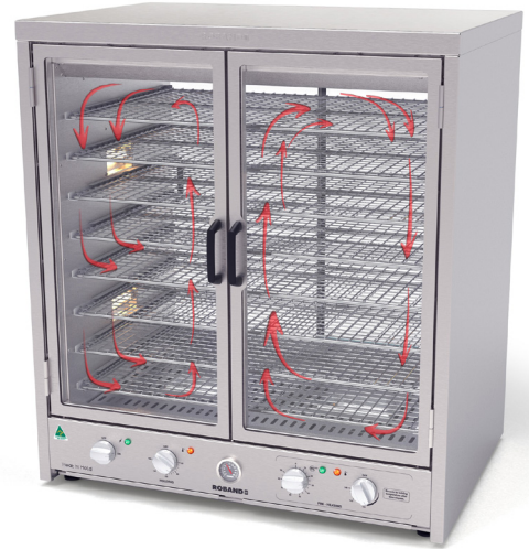
Control side of H200R depicting air flow propelled by dual fans throughout the cavity
