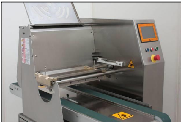
1. Lay the head on the supporting rods
