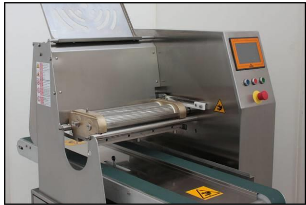
2. Delicately insert the two rollers
