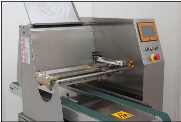
1. Lay the head on the supporting rods
