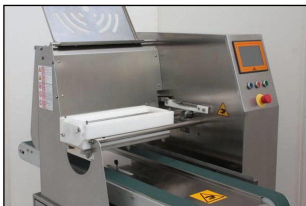
3. Position the front cap and fasten it using the relative stop nuts
