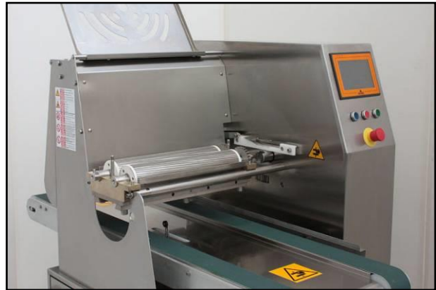
2. Delicately insert the two rollers
