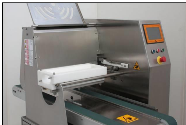
1. Lay the head on the supporting rods
