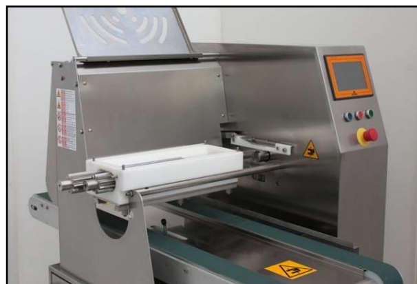
2. Delicately insert the two rollers into the cavity
