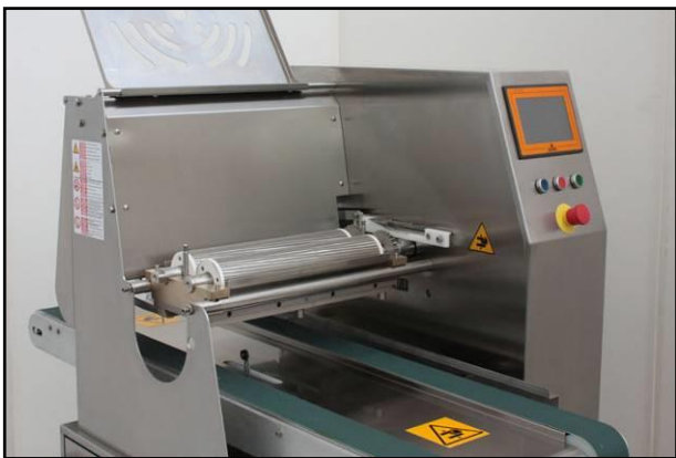
3. Carefully push the dosing group towards the structure, aligning the motor roller with the relative coupling
