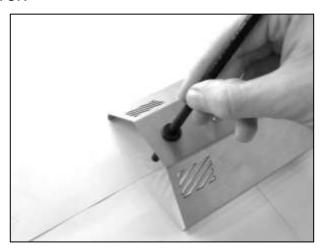
10) Install the heat lamp cover to the desired mounting location – screw / bolt the heat lamp cover to the mounting face as shown.
