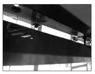
11) Reverse Steps 3 & 4 - Reinstall the heat lamp body into the cover and fasten the two flanged nuts with a 6 mm nut driver, taking care not to strip or bend the threaded tabs
