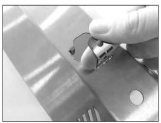
9) Re-insert the silicone grommet and PTFE sleeve so that approximately 20 mm of the PTFE sleeve extends into the cover.
