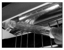
5) Using gentle force, push the lamp so that the sprung terminal pin and lamp end are compressed about 4mm. Rotate alternate end of lamp up into the terminal block taking care to line up Centre Pin of Lamp with Terminal Pin in terminal block. Release spring and allow lamp to seat between the two terminal blocks. Jiggle lamp slightly to make sure it is secure in place.
