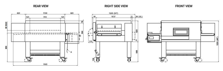
NOTE: The dimensions indicated in the views are in millimeters.
