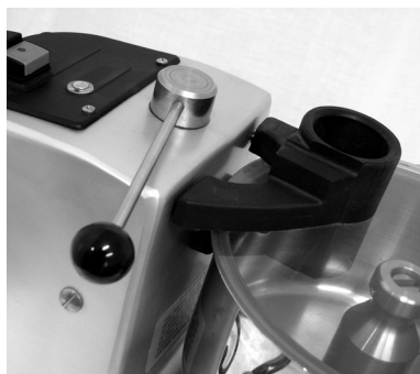
Safety interlocks prevent the machine operating if the clamping handle is not locked in place.
