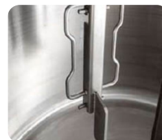
A performing mixing tool (unchanged form, patented) ensures an homogeneous mixing from top to bottom
