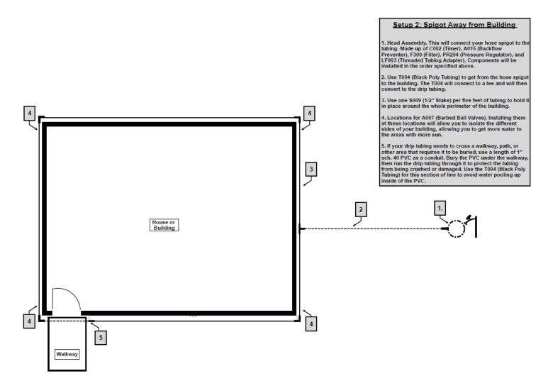
If you are planning to use a spigot away from your foundation for the medium or large size kit, use the LF009 at the end of the head assembly and run two separate lines of  $\frac{1}{2}$ " poly tube to the foundation instead of just one as shown above. This will ensure even watering of all sides of your foundation.
