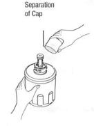
Align unlabeled area of filter with the indicator line so that it can be inserted into the filter cover. Turn the cartridge 1/4 turn to the right to lock it into place. You will feel a stop and the locked symbol should now be lined up with the indicator line.
