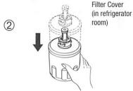
Apply the month sticker to the cartridge as a reminder to replace the filter within 6 months and remove red cap.
