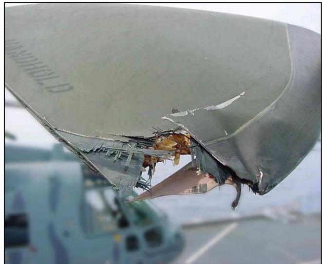
**Figure 6 - Tip Strike on AW101 Blade (Crown Copyright)**
