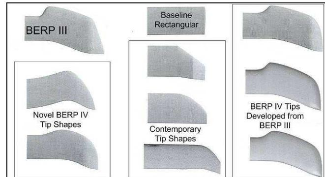
Figure 7 - Various Tip Shapes Assessed During BERP IV
