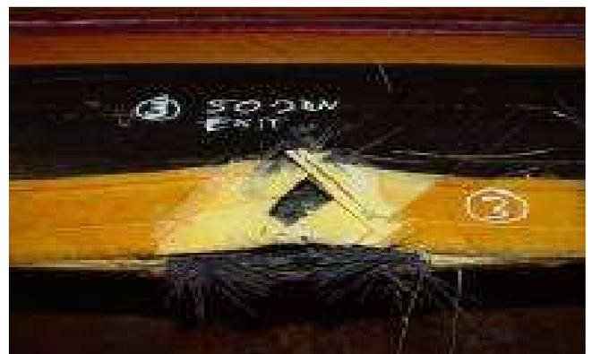
Figure 22 - Impacted Specimen
