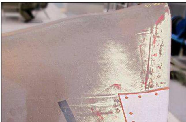
**Figure 5 - Sand Erosion on AW Lynx Blade Tip**
