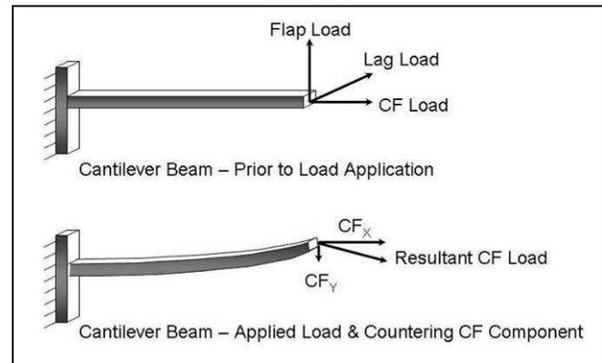
Figure 16 - Layout of Tradition Test Procedure
