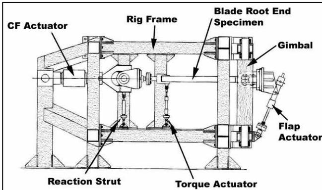
Figure 17 – Rig Side View
