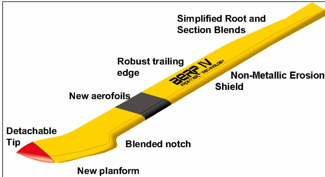
Figure 23 - Demonstrator Blade Features
