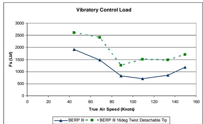
**Figure 13 - Predicted effect of Twist on Control Loads**
