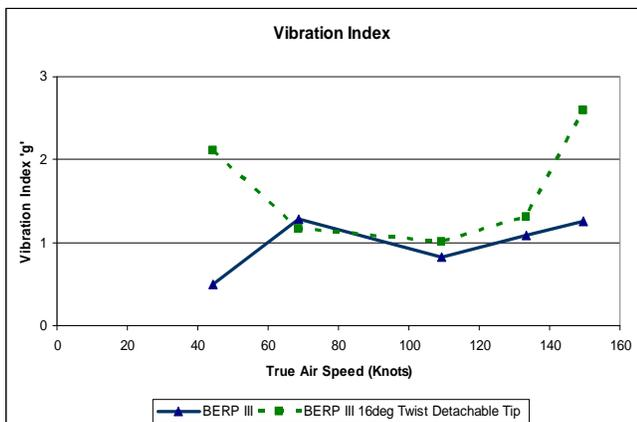
**Figure 12 - Predicted Effect of Twist on Vibration Index (ACSR Off)**
