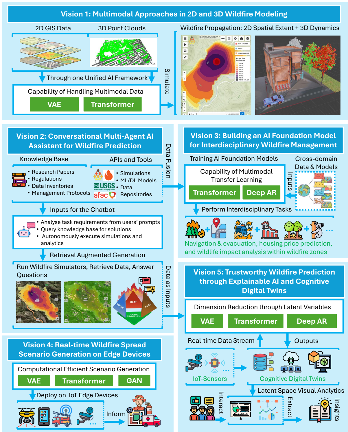
Figure 5: A summary of five future visions for applying generative AI to revolutionize wildfire prediction and management, ranging from the development of multimodal 2D and 3D wildfire modeling to the implementation of cognitive digital twins with explainable AI capabilities.
